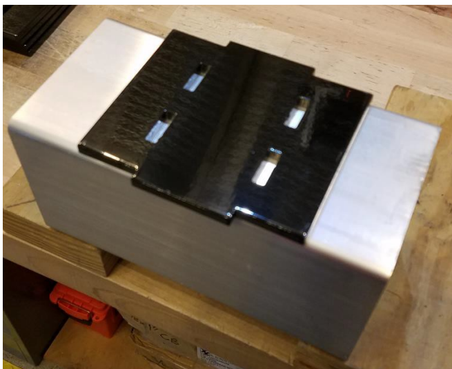
1. Set Base Plate on top of Bumper as shown.
