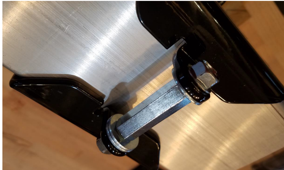
6. At opposite end of Face Plates, install Retention Fasteners. Use Coupling Nut, 2 Flange Bolts, and 1 Flat Washer at each end (ignore 2 Flat Washers shown at far end of Coupling Nut). Finger-tighten bolts for now.
