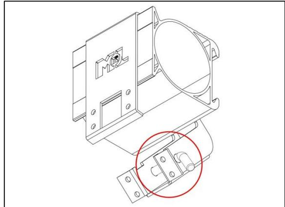
**Step 5:** Swing faceplate out slightly and swing flanged channel up until almost tight to bottom side of bumper.
