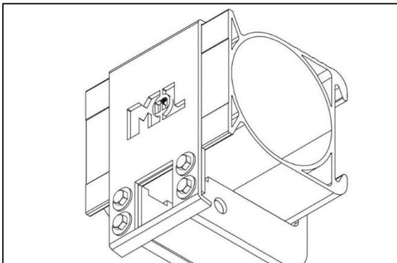
Last Step: Your Mount-n-Lock™ 2-Inch Hitch Receiver includes at no additional charge a saddle clamp which can be used to reduce the rattle of your hitch accessories. The following cut-away view of just the flanged channel and the saddle clamp shows how the saddle clamp is installed once your hitch accessory is in the hitch receiver.
