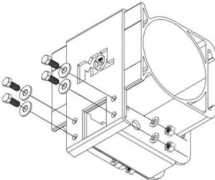
Step 8: Use torque wrench to tighten bolts to 44 ft. lbs. of torque. Your Mount-n-Lock™ 2-Inch Hitch Receiver is now ready to use!
