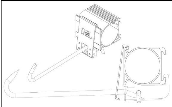
Step 7: With channel's flange nested atop the faceplate's lower lip, remove crowbar and insert 3/8" x 1" bolts as shown.
