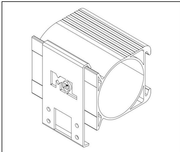
**Step 3:** Hang flanged channel from rear lip of bumper so that it aligns with faceplate.
