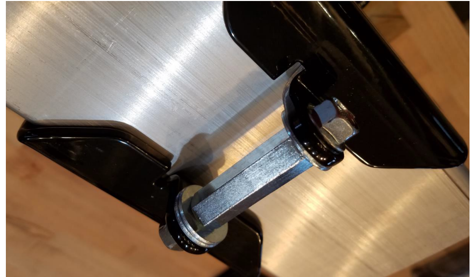
6. At opposite end of Face Plates, install Retention Fasteners. Use Coupling Nut, 2 Flange Bolts, and 1 Flat Washer at each end (ignore 2 Flat Washers shown at far end of Coupling Nut). Finger-tighten bolts for now.
